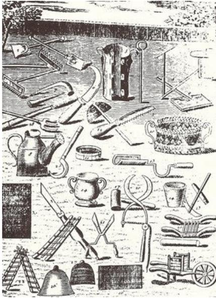
**1 Spade.** The first instrument the Gardener takes in his hand to learn a dexterity in turning up the Ground and working it smooth and even and it is chiefly used by Apprentices.
